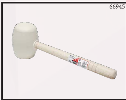
Rubber Hammer to pound tile while laying to ensure uniform spread of adhesive underneath.
